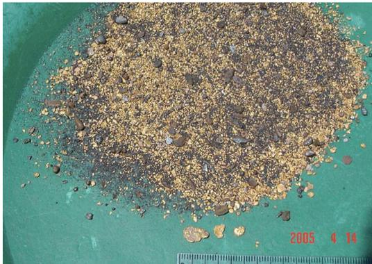
Previous sampling at the deposit has included rudimentary gold panning tests, and larger scale bulk sampling using standard gravity recovery plants. The most recent sampling prior to Pacific Niugini involvement was by Resource Development Inc. of Colorado, who reported an average feed grade of 0.57 g/t for a 950kg bulk sample.
