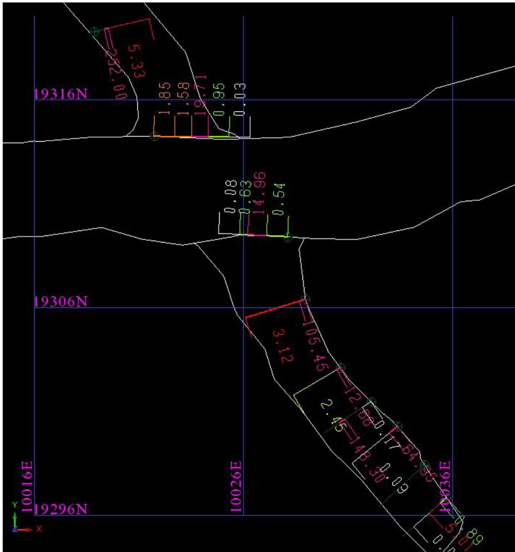
Figure 4 - 2215 Level High grade ore development with Face grades in the Bobby Lode outside of the current Mineral Resource estimate.
