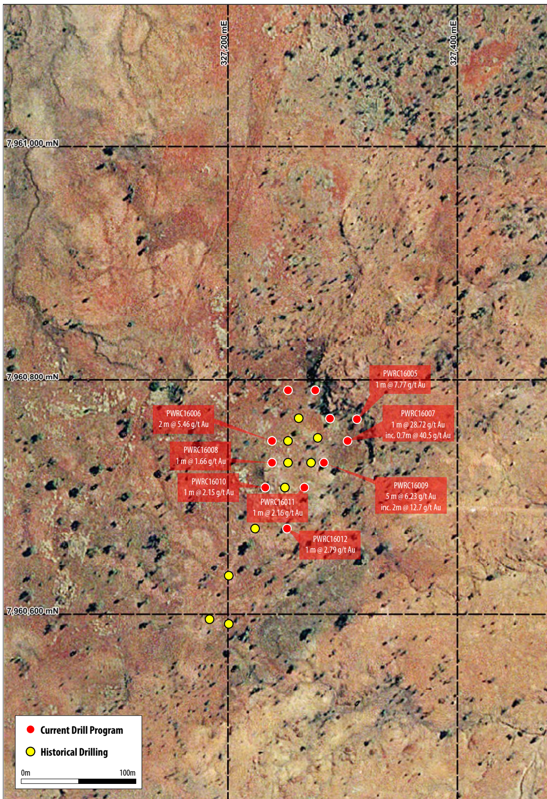
Figure 1: Paddock Well drilling location plan showing significant intersections from the current drilling program.
