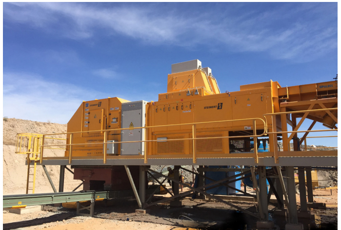
Ore Sorter in operation
