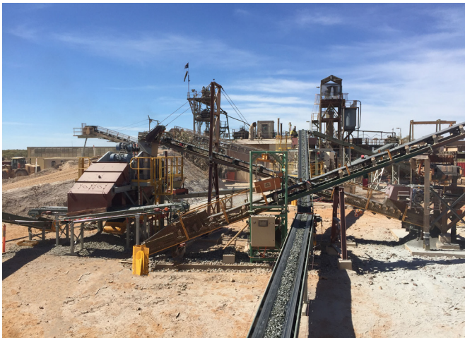
Ore Sorter product belt feeding tertiary crusher
